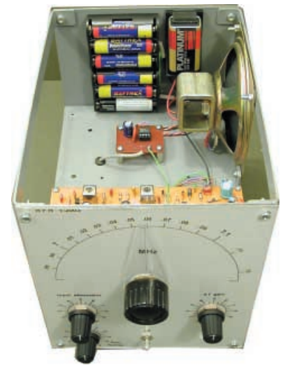
The two separate power supply battery "packs", one for the receiver and the other for the amplifier, located on the rear panel.
