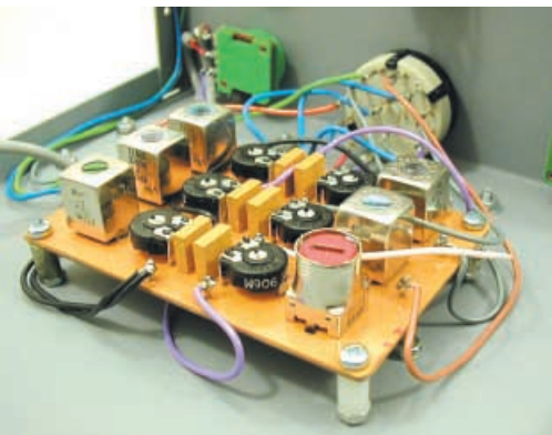
General Coverage coil pack p.c.b. wired to the wavechange switch.
