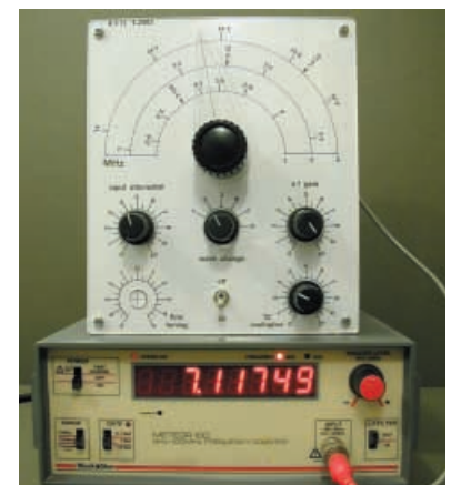
A frequency counter wired, via the Buffer Amplifier, to the Regenerative Radio and showing an amateur band frequency readout.
