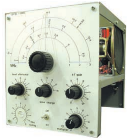
Fig.4.9. Calibrated dial (half-size approx.) for the Amateur Bands Receiver. Typical frequency "markers" are indicated by the arrowhead pointers.
