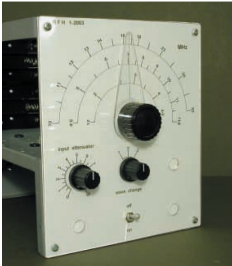
Fig.7.12. Calibrated tuning dial (half-size approx.) for the 3-Band SW Superhet Tuner.
