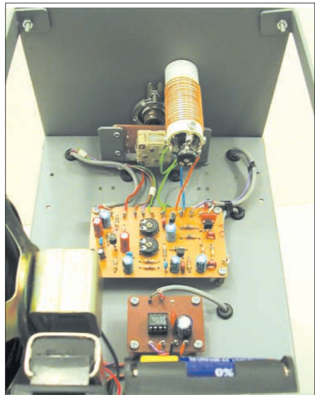
General layout inside the metal case. The speaker amplifier module is in the foreground. The wave trap is mounted on the underside boxed chassis.
